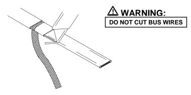
**4** Shave the core material from the outside of each bus wire.
