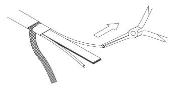
Starting at the end, in the same plane as the cable, pull each bus wire away from the core material.
