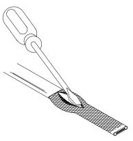
**3** At the bulge, separate the braid to make an opening.
