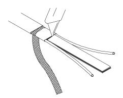
6 Remove the exposed core material.
