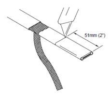
• Lightly cut around the heater outer jacket 51mm (2") from the end. Bend the cable to break outer jacket.
