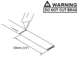
• Lightly cut around the cable overjacket 89mm (3.5") from the end. Bend cable to break the overjacket.
