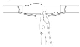
If necessary, cut excess length from braid straps. Crimp the braid straps together into an uninsulated splice connector. Secure the connector at the indented area with one and a half wraps of fiberglass tape (not included in kit).
