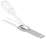
**5** At the bulge, separate the braid to make an opening.
