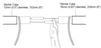
2 Slide one 13mm (0.5") diameter, 152mm (6") length shrink tube over one of the heater cables. Crimp an insulated splice connector to each bus wire connecting the two heater cables together.
