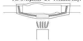
**6** Center the 16mm (0.63") diameter, 229mm (9") length shrink tube over the splice and braid connection. Shrink with heat gun until completely shrunk. A uniform bead of glue should appear around the ends of the shrink tube.
