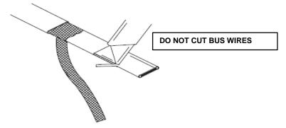
**4** Shave the core material from the outside of each bus wire.
