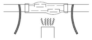
2 Center the 13mm (0.5") diameter, 152mm (6") length shrink tube over the connectors leaving the braid straps exposed. Shrink with heat gun until completely shrunk. A uniform bead of glue should appear around the ends of the shrink tube.
