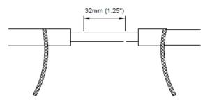
• Position both heater cables with the ground braid on the same side. Remove 32mm (1.25") of bus wire from each heater cable to offset for insulated splice connectors.
