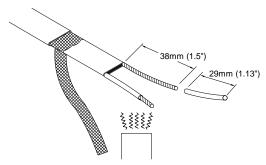
• Slide a 3mm (.125") ID shrink tube over each bare bus wire and shrink with an industrial heat gun or rapidly moving fluffy flame.
