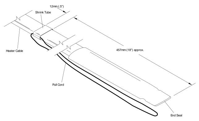
Install the nylon pull cord through the shrink tube and tie the ends together. (The pull cord length should be approx. 2m (6.6') long.)
