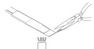
Place the second layer of shrink tube over the end seal and shrink with an industrial heat gun or rapidly moving fluffy flame. Allow approx.
