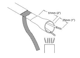
Slide the 12mm (0.5") ID shrink tube over both wires, 25mm (1") of each bus wire should be exposed. Shrink with an industrial heat gun or rapidly moving fluffy flame until completely shrunk.
