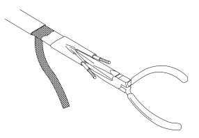
• While still warm, spread pigtail wires and squeeze with needle-nose pliers.
