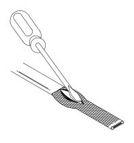
Lightly cut around heater overjacket 127mm (5") from the end. Bend cable to break the overjacket.
