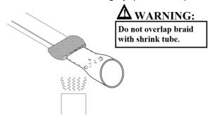
Slide a 51mm (2") length shrink tube over the heater cable leaving 25mm (1") of shrink tube past the heater cable. Shrink with heat gun until completely shrunk.
