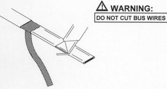
**4** Shave the core material from the outside of each bus wire.
