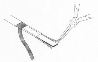
Starting at the end, pull each bus wire away from the core material.
