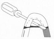
**6** While bending heater cable, work it through the braid opening.
