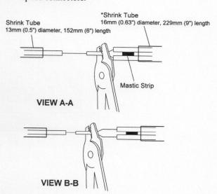
2 Slide one 13mm (0.5") diameter, 152mm (6") length shrink tube over the single heater cable side. Twist bus wires together from the two heater cables and crimp into insulated splice connectors, then connect to the single heater cable. Place a mastic strip between the two heater cables forming a moisture harrier.
