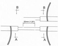
Position three heater cables with the ground braid on the same side. Remove 32mm (1.25") of bus wire from each heater cable to offset for the insulated splice connectors.
