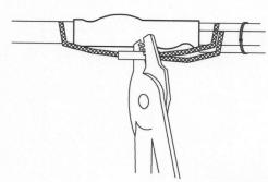
If necessary, cut excess length from braid straps. Crimp the braid straps together into an uninsulated splice connector. Secure connector at the indented area with one and a half wraps of fiberglass tape (not included in kit).
