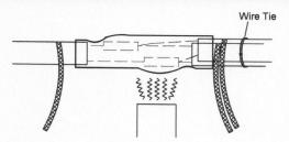
3 Center the 13mm (0.5") diameter, 152mm (6") length shrink tube over the connectors leaving the braid straps exposed. Make sure the shrink tube covers the mastic strip. Shrink with heat gun until completely shrunk. A uniform bead of glue should appear around the ends of the shrink tube. Fasten a wire tie around the two heater cables to hold in place.
