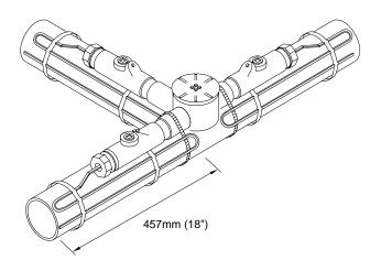
• Allow 457mm (18") of heater cable for each side to compensate for heat loss of the termination kit.
