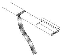
3 Remove the jacket from the heater cable.
