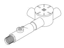
Thread the reducer bushing into the junction box. Then thread the male adapter into the reducer bushing. Finally, thread the seal fitting into the male adapter. Tighten to a minimum of 5 full threads of engagement.
