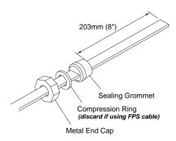
Slide a metal end cap, \*compression ring and sealing grommet over each heater cable. Position each sealing grommet 203mm (8") from each cable end.
