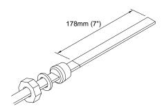
**6** Prepare all heater cables for termination. Proceed to "Overjacket Stripping Procedures", sheet 3 of 8
