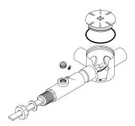
Remove box cover and box cover gasket from junction box, place a power termination through each cable entry seal and seal fitting. Slide forward until the sealing grommet is flush with the entry seal.
