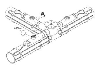
Center a heater cable inside each conduit opening. Using the X fiber, pack around each heater cable forming a dam to hold the sealing compound.
